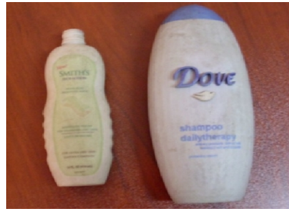
(Figure 1-f- Samples of colored packages printed by Z printer- powder type zp150 Figure 1: An example of jet processes
