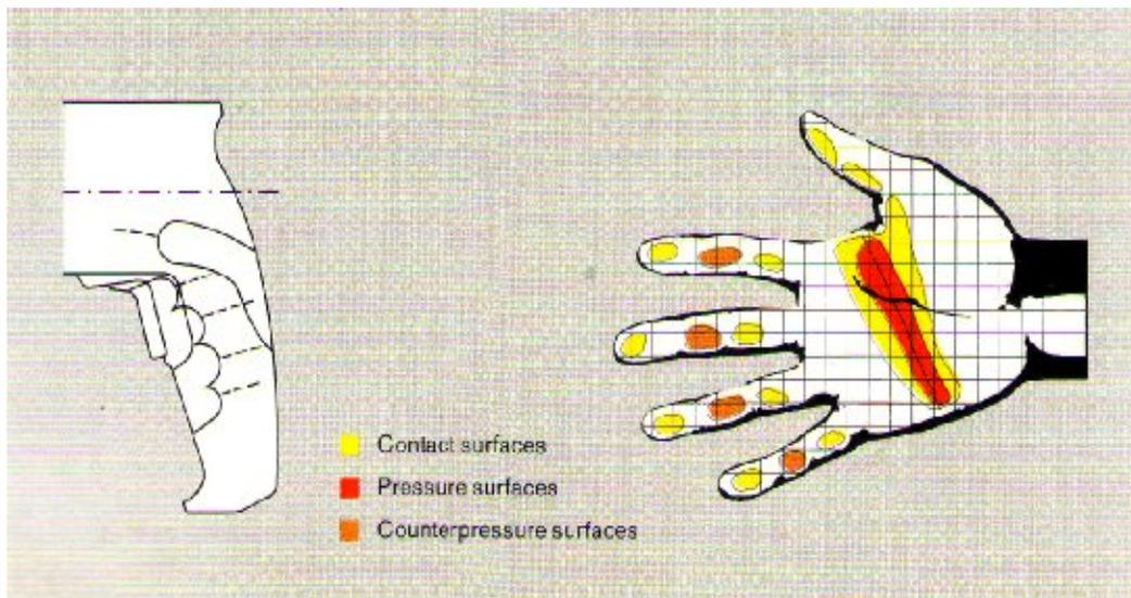
Figure (2) Three surfaces affected by gripping
