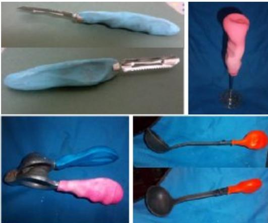
Figure (13) some of the kitchen tools with handles modified
