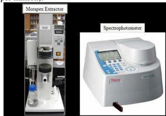
Figure 2: Photo showing Japanese test method 112 Extractor and spectrophotometer Released Formaldehyde is determined using AATCC Test Procedure 112 (Durbin Extraction). It is called a Sealed Jar Method providing an analytical means for determining the amount of formaldehyde released under the condition of accelerated storage. Simulated released formaldehyde – breathing exposure, uses an incubator, sealed jar and water bath which is then read on a spectrophotometer, as shown in Figure
