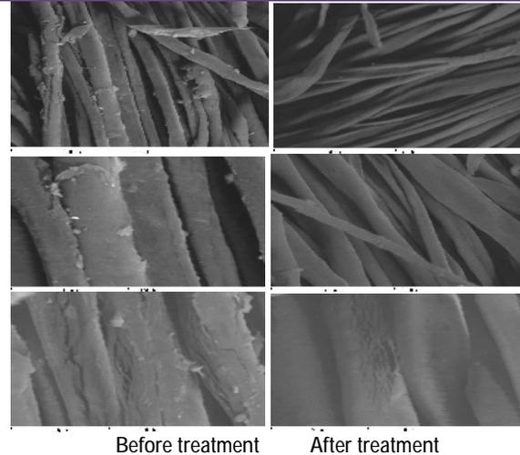
Fig.(5) Scanning electron measurements for the fabric before and after treatment using a scanning electron microscope (SEM)
