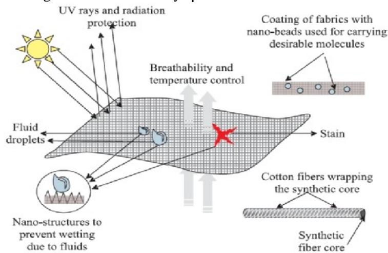
Fig.(2) Fabric finishing for functional properties and performance. (2)
