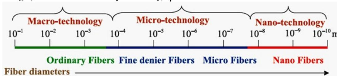
Fig.(1) Fiber size and associated manufacturing technologies.<sup>(2)</sup>
