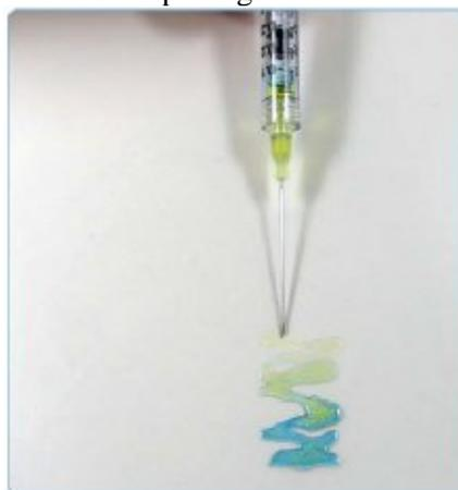
Figure 13: Demonstration of indicator color change after exposure to oxygen
