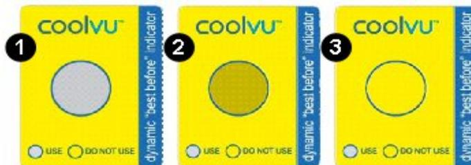
Figure 6: CoolVu labels, a - freshly activated label, b - mid-life label, c - expired label
