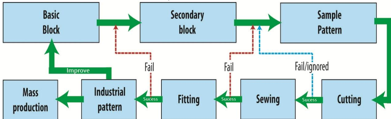
Figure (3) the suggested prototype developing method (Each process' errors fixed internally)
