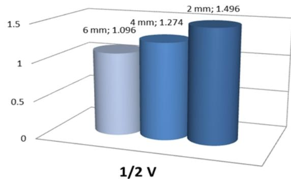
Fig. (7): The relationship between the Pile height mm & Fire Area cm<sup>2</sup> at constant of Weave Structure of Pile (1/2 V)
