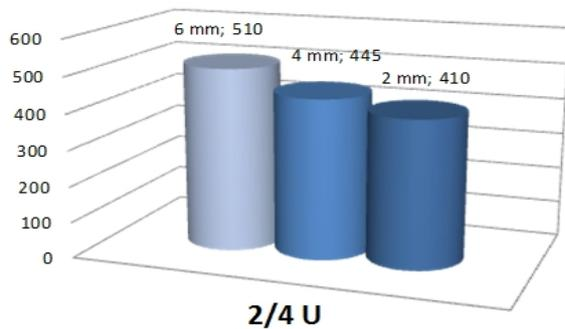
Fig. (5): The relationship between the Pile height mm & Fabric Weight g/m<sup>2</sup> at constant of Weave Structure of Pile (2/4 U)
