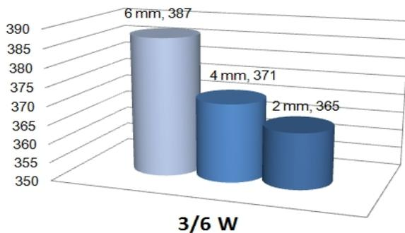
Fig. (6): The relationship between the Pile height mm & Fabric Weight g/m<sup>2</sup> at constant of Weave Structure of Pile (3/6 W)
