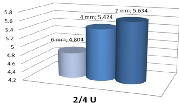
Fig. (8): The relationship between the Pile height mm & Fire Area cm<sup>2</sup> at constant of Weave Structure of Pile (2/4 U)
