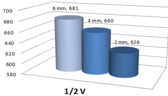
Fig. (4): The relationship between the Pile height mm & Fabric Weight g/m<sup>2</sup> at constant of Weave Structure of Pile (1/2 V)
