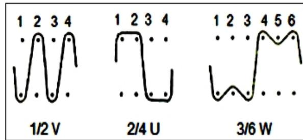
Fig. (3): Pile structure (1/2V, 2/4U, 3/6W)
