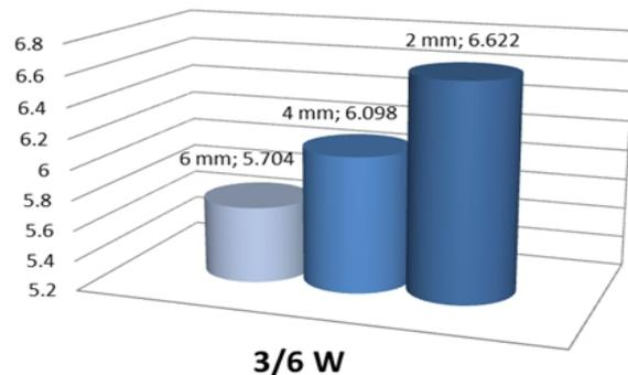
Fig. (9): The relationship between the Pile height mm & Fire Area cm<sup>2</sup> at constant of Weave Structure of Pile (3/6 W)
