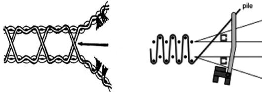
Fig. (1): Face to face weaving principle
