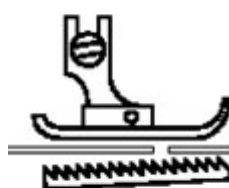
(b) Position of the feed dog with its side opposite the operator in a lowered position.
