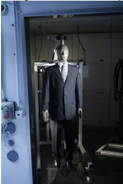
Figure 8. Sherlock thermal manikin
