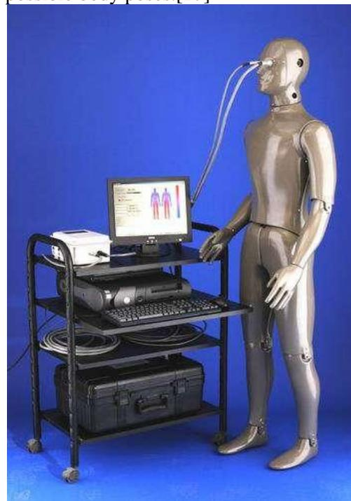
Figure.1 "Newton" thermal manikin
