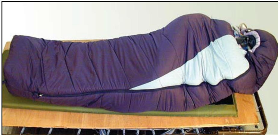
Figure 4: The articulated manikin, "Charlie 3", measures the thermal insulation of sleeping bags
