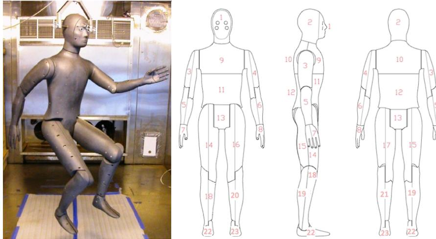
Figure 3. NEMO 23-zone submersible thermal manikin.
