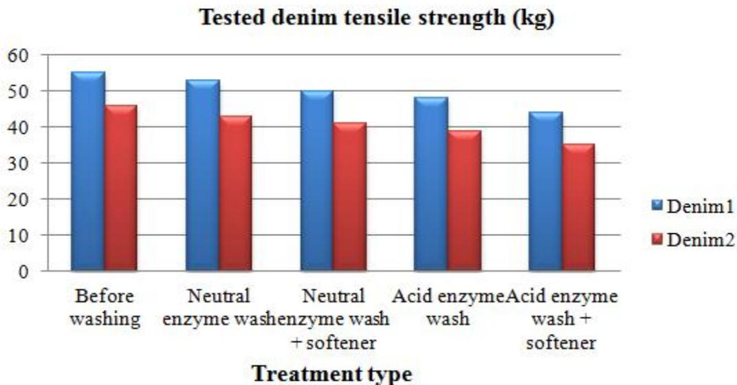
Fig.6: Tested denim tensile strength before washing, after washing and after softening
