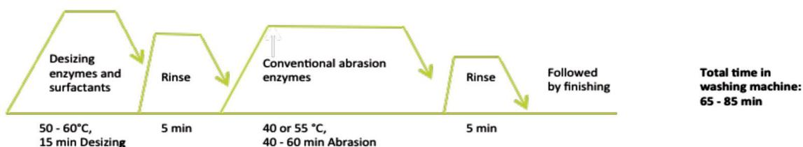
Fig.2: Denim enzyme washing process flow chart <sup>(9)</sup>
