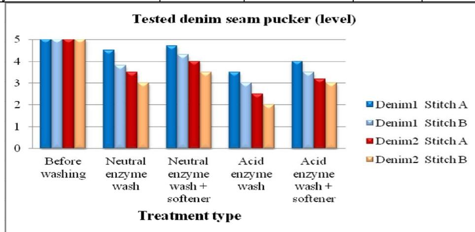
Fig.10: Tested denim seam pucker before washing, after washing and after softening
