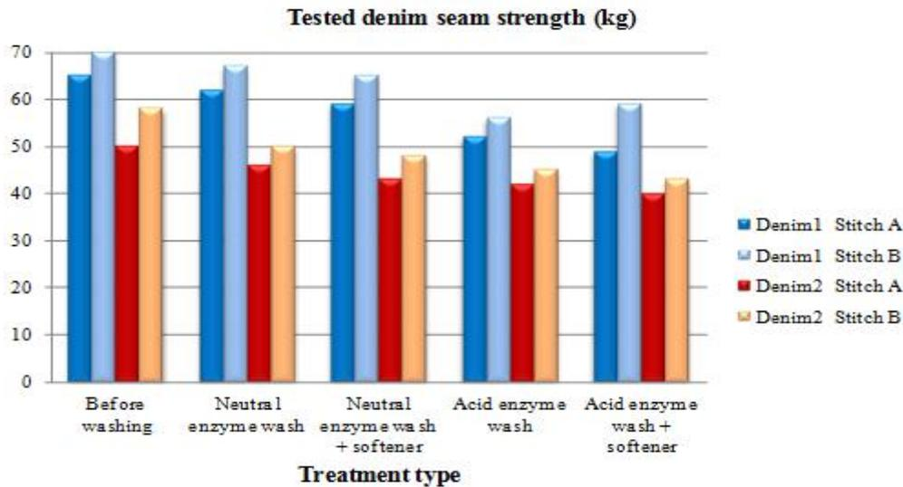
Fig.9: Tested denim seam strength before washing, after washing and after softening
