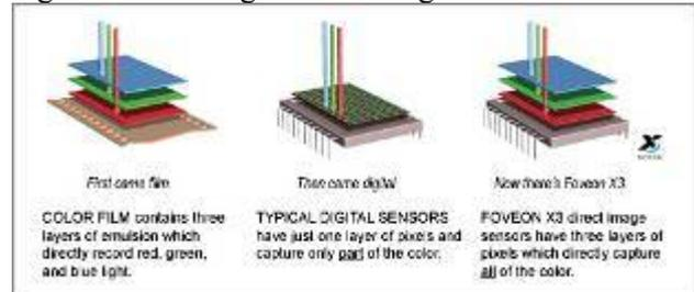
**Fig (38) show the difference between Foveon image sensor and the Typical digital sensor.**
