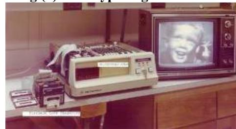
**Fig (3) Prototype Digital Camera Playback system.**
