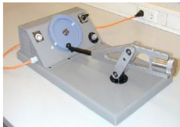
Figure 3. “Aachen Felting Test“ and is used to felting property of loose wool and determine the combed top.
