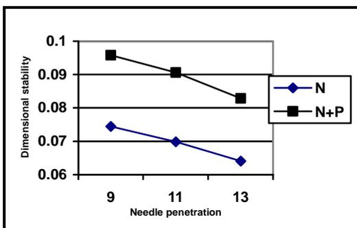
Fig. (23) Effect of fabric type and needle penetration depth mm on the dimensional stability(shrinkage of fabric ratio % in both direction) at weight 3400 gm/m<sup>2</sup>
