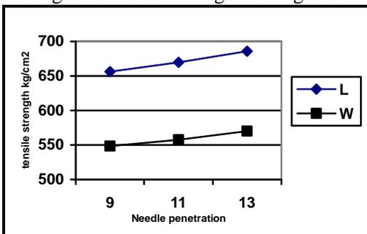
Fig. (5) Effect of fabric type and needle penetration depth mm on the tensile strength at break in the two directions of the fabric type 100% Nomex at weight 3400 gm/m<sup>2</sup>
