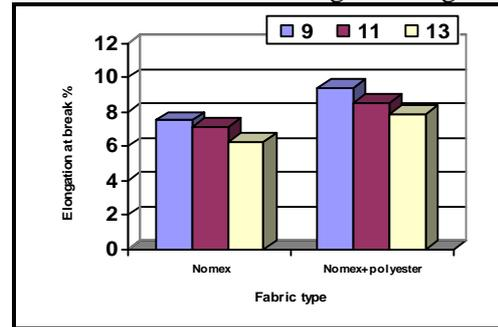
Fig. (12) Effect of fabric type and needle penetration depth mm on the elongation at break % in the width direction at weight 3150 gm/m<sup>2</sup>
