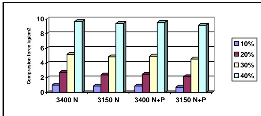
Fig. (19) Effect of fabric type and the weight gm/m<sup>2</sup> on the compression force kg/cm<sup>2</sup>(lost of thickness ratio %) at puncture depth 9 mm
