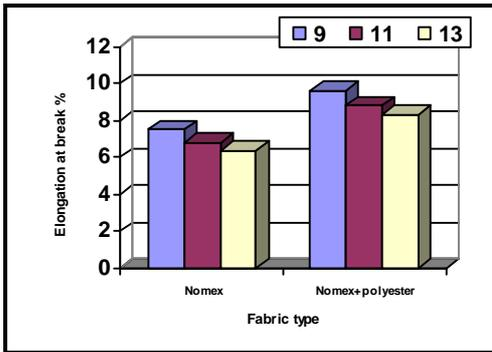
Fig. (9) Effect of fabric type and needle penetration depth mm on the elongation at break % in the length direction at weight 3400 gm/m<sup>2</sup>
