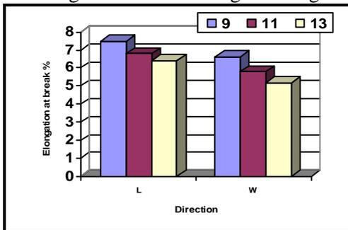
Fig. (13) Effect of fabric type and needle penetration depth mm on the elongation at break % in the two directions of the fabric type 100% Nomex at weight 3400 gm/m<sup>2</sup>
