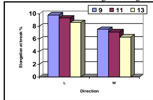
Fig. (14) Effect of fabric type and needle penetration depth mm on the elongation at break % in the width direction of the fabric type 100% Nomex at weight 3150 gm/m<sup>2</sup>
