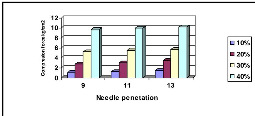
Fig. (22) Effect of needle penetration depth mm on the compression force kg/cm<sup>2</sup> (lost of thickness ratio %) at weight 3400 gm/m<sup>2</sup> of 100% Nomex fabric type
