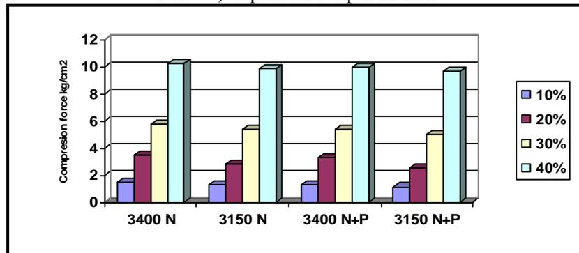
Fig. (21) Effect of fabric type and the weight gm/m<sup>2</sup> on the compression force kg/cm<sup>2</sup>(lost of thickness ratio %) at puncture depth 13 mm
