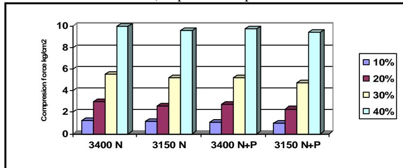
Fig. (20) Effect of fabric type and the weight gm/m<sup>2</sup> on the compression force kg/cm<sup>2</sup>(lost of thickness ratio %) at puncture depth 11 mm
