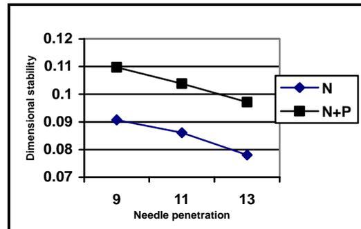
Fig. (24) Effect of fabric type and needle penetration depth mm on the dimensional stability(shrinkage of fabric ratio % in both direction) at weight 3150 gm/m<sup>2</sup>
