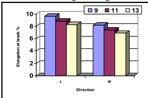
Fig. (15) Effect of fabric type and needle penetration depth mm on the elongation at break % in the two directions of the fabric type 75% Nomex + 25% polyester at weight 3400 gm/m<sup>2</sup>
