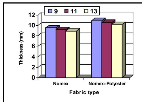
Fig. (26) Effect of fabric type and needle penetration depth mm on the thickness (mm) at weight 3150 gm/m<sup>2</sup>
