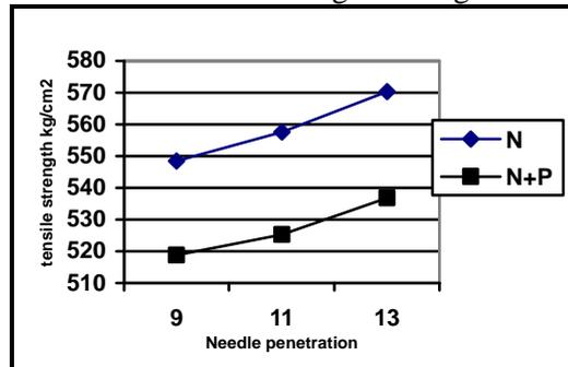
Fig. (4) Effect of fabric type and needle penetration depth mm on the tensile strength at break in the width direction at weight 3150 gm/m<sup>2</sup>
