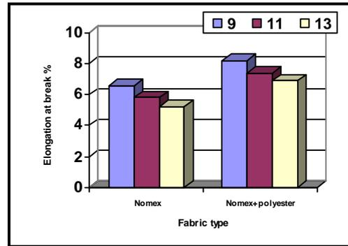
Fig. (10) Effect of fabric type and needle penetration depth mm on the elongation at break % in the width direction at weight 3400 gm/m<sup>2</sup>
