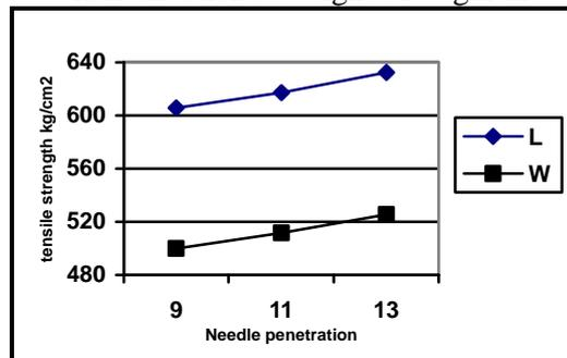
Fig. (6) Effect of fabric type and needle penetration depth mm on the tensile strength at break in the two directions of the fabric type 100% Nomex at weight 3150 gm/m<sup>2</sup>
