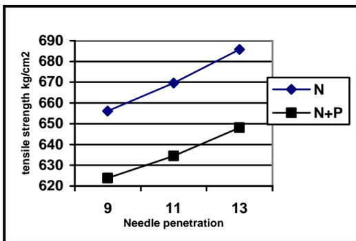
Fig. (1) Effect of fabric type and needle penetration depth mm on the tensile strength at break in the length direction at weight 3400 gm/m<sup>2</sup>
