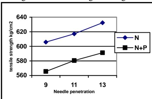
Fig. (3) Effect of fabric type and needle penetration depth mm on the tensile strength at break in the length direction at weight 3150 gm/m<sup>2</sup>
