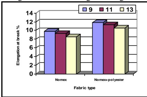
Fig. (11) Effect of fabric type and needle penetration depth mm on the elongation at break % in the length direction at weight 3150 gm/m<sup>2</sup>
