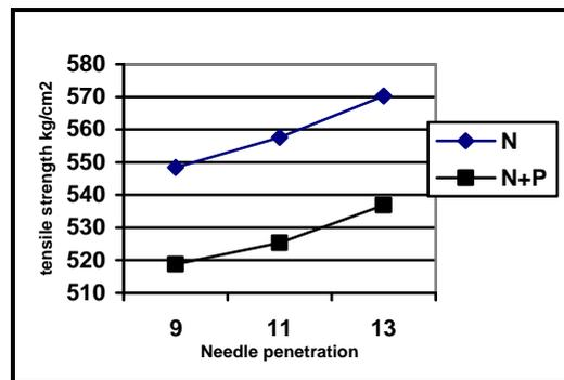
Fig. (2) Effect of fabric type and needle penetration depth mm on the tensile strength at break in the width direction at weight 3400 gm/m<sup>2</sup>
