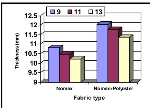
Fig. (25) Effect of fabric type and needle penetration depth mm on the thickness (mm) at weight 3400 gm/m<sup>2</sup>
