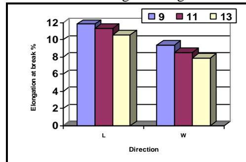
Fig. (16) Effect of fabric type and needle penetration depth mm on the elongation at break % in the two directions of the fabric type 75% Nomex + 25% polyester at weight 3150 gm/m<sup>2</sup>
