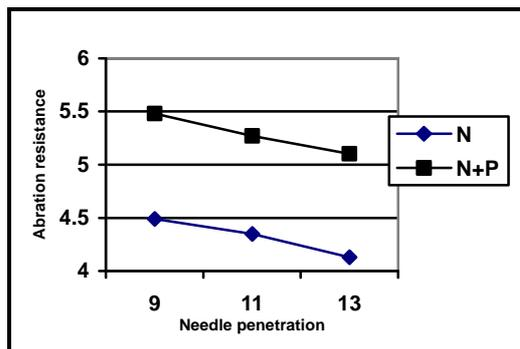
Fig. (17) Effect of fabric type and needle penetration depth mm on the abrasion resistance (lost weight ratio% at 2000 cycle) at weight 3400 gm/m<sup>2</sup>
