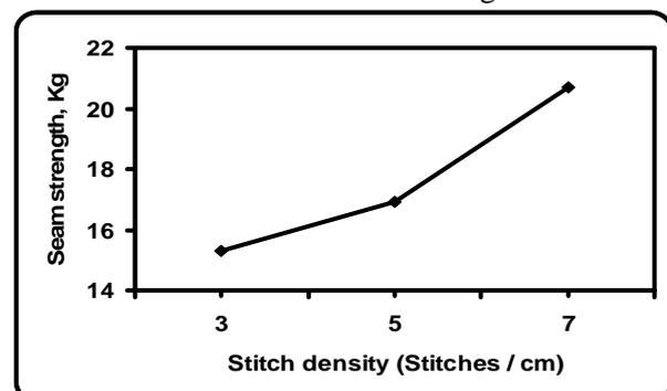
Figure 8: Effect of stitch density on seam strength
