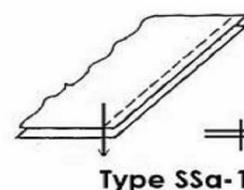
Figure 1: Supper imposed seam of type SSa-1
