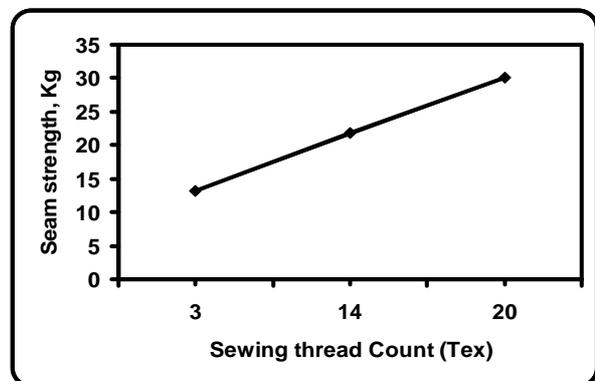
Figure 5: Effect of sewing thread count on seam strength
