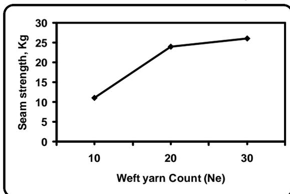
Figure 4: Effect of weft yarn count on seam strength
