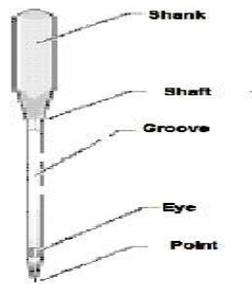
Figure 2: General view of sewing needle
