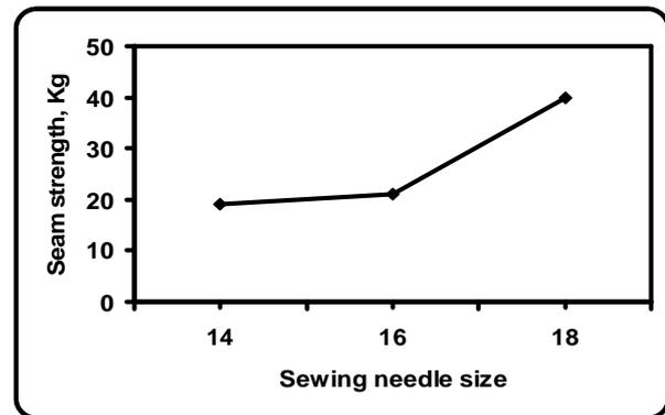
Figure 7: Effect of sewing needle size on seam strength
