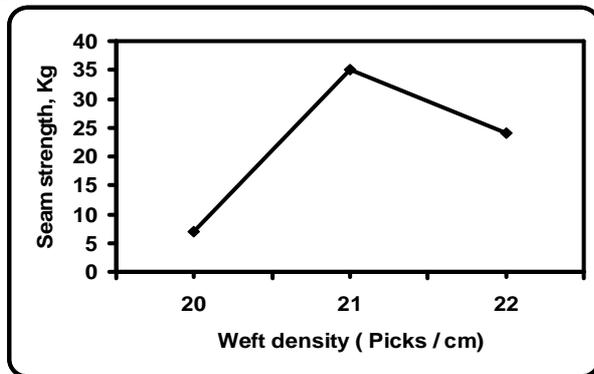
Figure 6: Effect of weft density on seam strength
