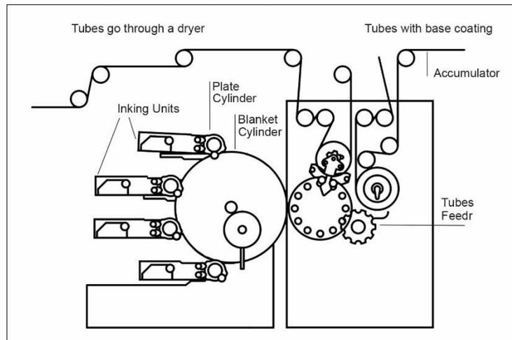
**Figure 2:** Rotary dry offset letterpress machine structure
