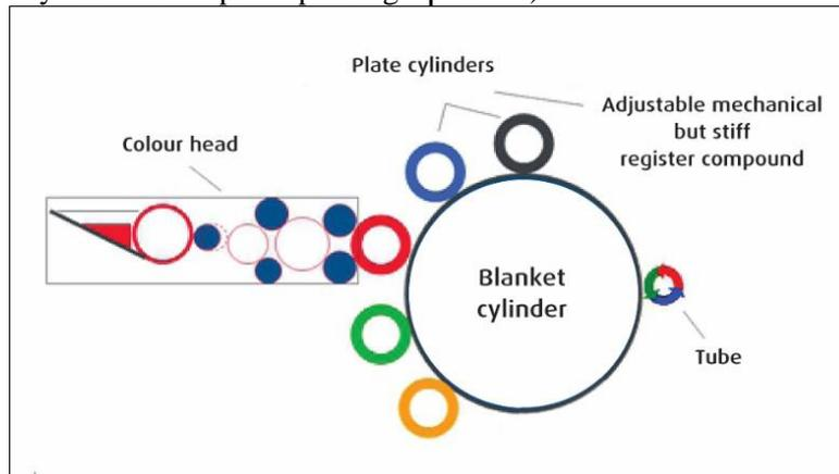
**Figure 1:** The principle of dry offset letterpress printing
