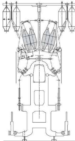
Fig (1): Formation of dual core yarn with welding.
